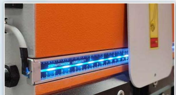
Shows the location of the bent pieces and bending stations with coloured LED bars.
