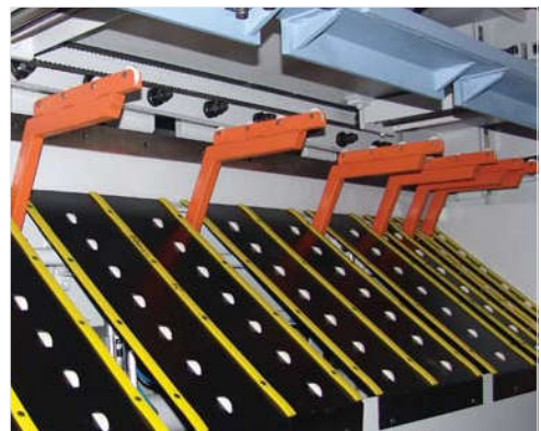
■ Sheet metal being cut can slide with minimum scratch thanks to rollers and bearings on lever type pneumatic sheet metal support system (O)
