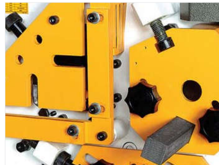
■ Bar cutting station
