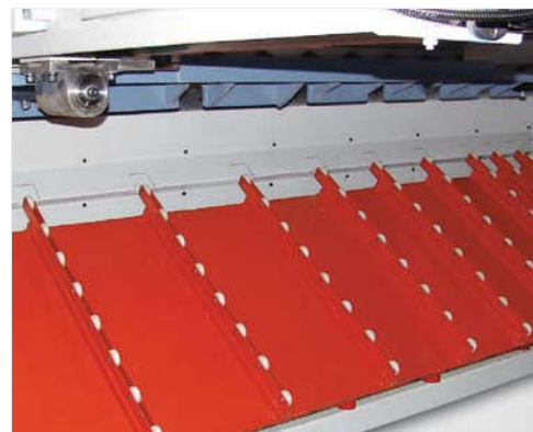
■ Mono-block type pneumatic sheet metal support system prevents hanging down wide and thin sheet metal to enable more precise cutting (O)
