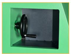
The handle for adjustment of the material thickness on the upper beam is nice hidden away in the gable - again to have nice clean surfaces and at the same time protect the handle.
