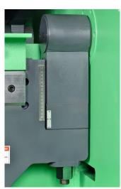
Adjustment of the material thickness on the bending bend is easy with a mm scale.
