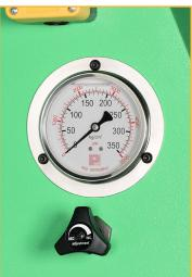
The HBM folders offer adjustment of the hydraulic pressure to match the material thickness - so no damage to the material surface is avoided.
